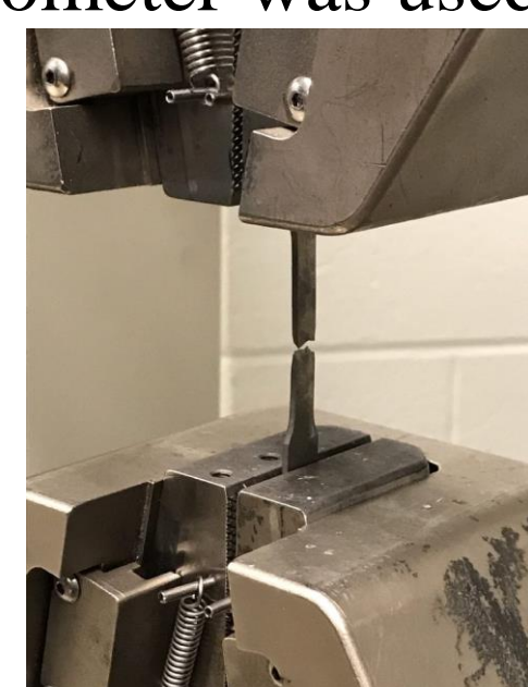
Figure 6 | Fractured sample in the MTS tensile machine.
